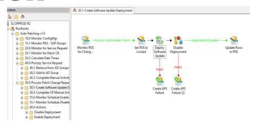
The Solution enables SCCM to raise patch deployment failures as SCOM Alerts, so it is immediately obvious which devices require patch remediation.
